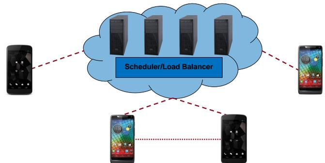
Fig. 1. Existing offloading scenarios where computation can be offloaded to cloud computing services or neighboring mobile devices
